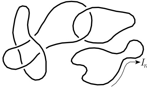
FIGURE 26: Current-carrying loops interact magnetically. We are not concerned at the moment with the mechanism (batteries?) that in reality would be required to maintain the steady currents I_n .
